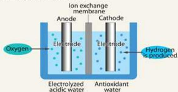
Electrolysis is a process whereby an electric current is passed through water containing an electrolyte (a mineral ion, for example), causing oxidation and reduction reactions that would not otherwise have occurred. The water on the anode side is oxidized and the water on the cathode side is reduced, thus antioxidant water is produced.
